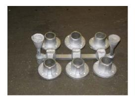
3. The raw castings from the foundry then pass through several processing and finishing stages to become the final product as shown below.
