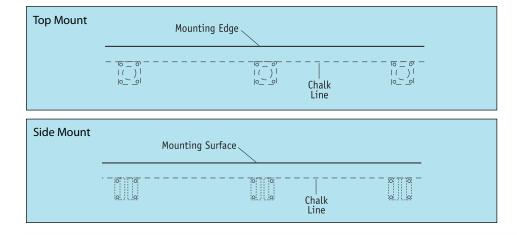
Flanges should be aligned along the chalk line and spaced the distance shown on project drawings. Drill holes in concrete using flange as a template and install anchors per manufacturers' recommendation.
